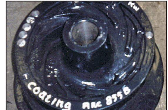
Coated impeller awaiting installation in submersible pump
