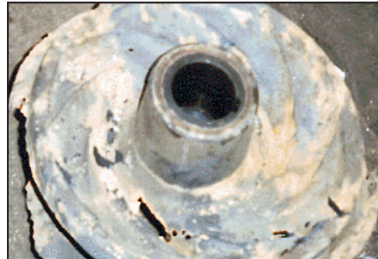
Corroded impeller from submersible pump
